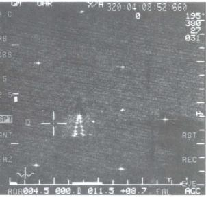
AN/APG-76 real-time, on-board 3-foot (top) and 1-foot (bottom) SAR imagery of an array of radar reflectors at Wolf-Webster Air Field. The individual reflectors are 3 feet apart at the apex and are clearly resolved by the radar. The range to the target is over 30 nmi. Note the shadow of trees in lower right.
