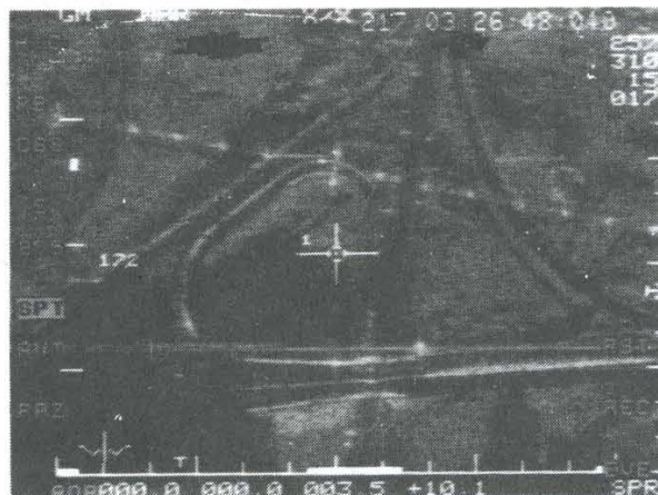
On-board 1-meter resolution SAR map of an area near Baltimore-Washington International Airport. In addition to the "cloverleaf" intersection of Route 170 and I-195, the approach lights to BWI runways are clearly visible. The image was made at a range of 31 km.
