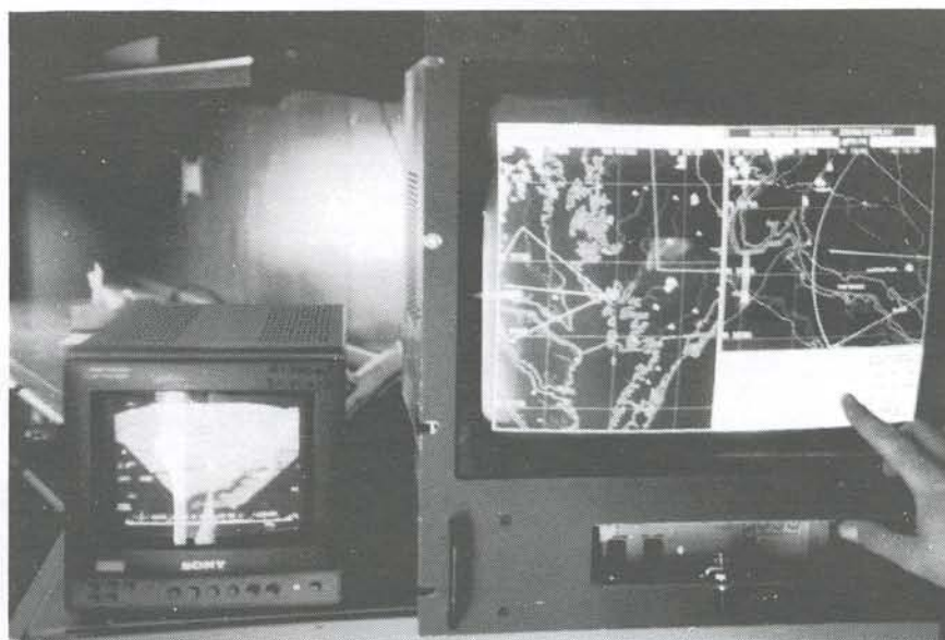
The Situation Station Displays Map Based Information Relative to Real-Time Aircraft and Target Geometries.
